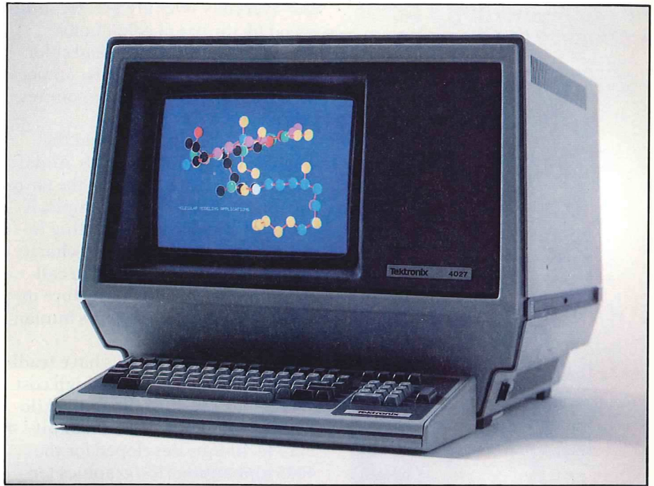
Fig. 1. The 4027 Color Graphics Terminal. A molecular modeling application is displayed.
